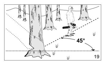
Then, establish a path of escape and remove all obstacles. This path should be opposite to the planned direction of the fall of the tree and at a 45° angle (fig. 19). An alternate path must also be selected. Place all tools and equipment a safe distance away from the tree, but not on the escape path.
